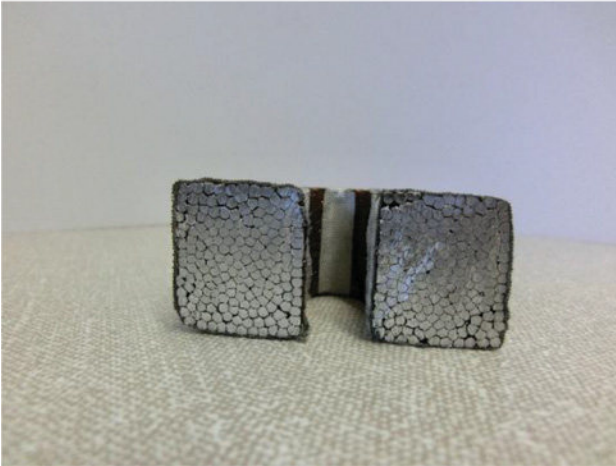
Figure 4.1 Pressed coil for high slot fill factor.
